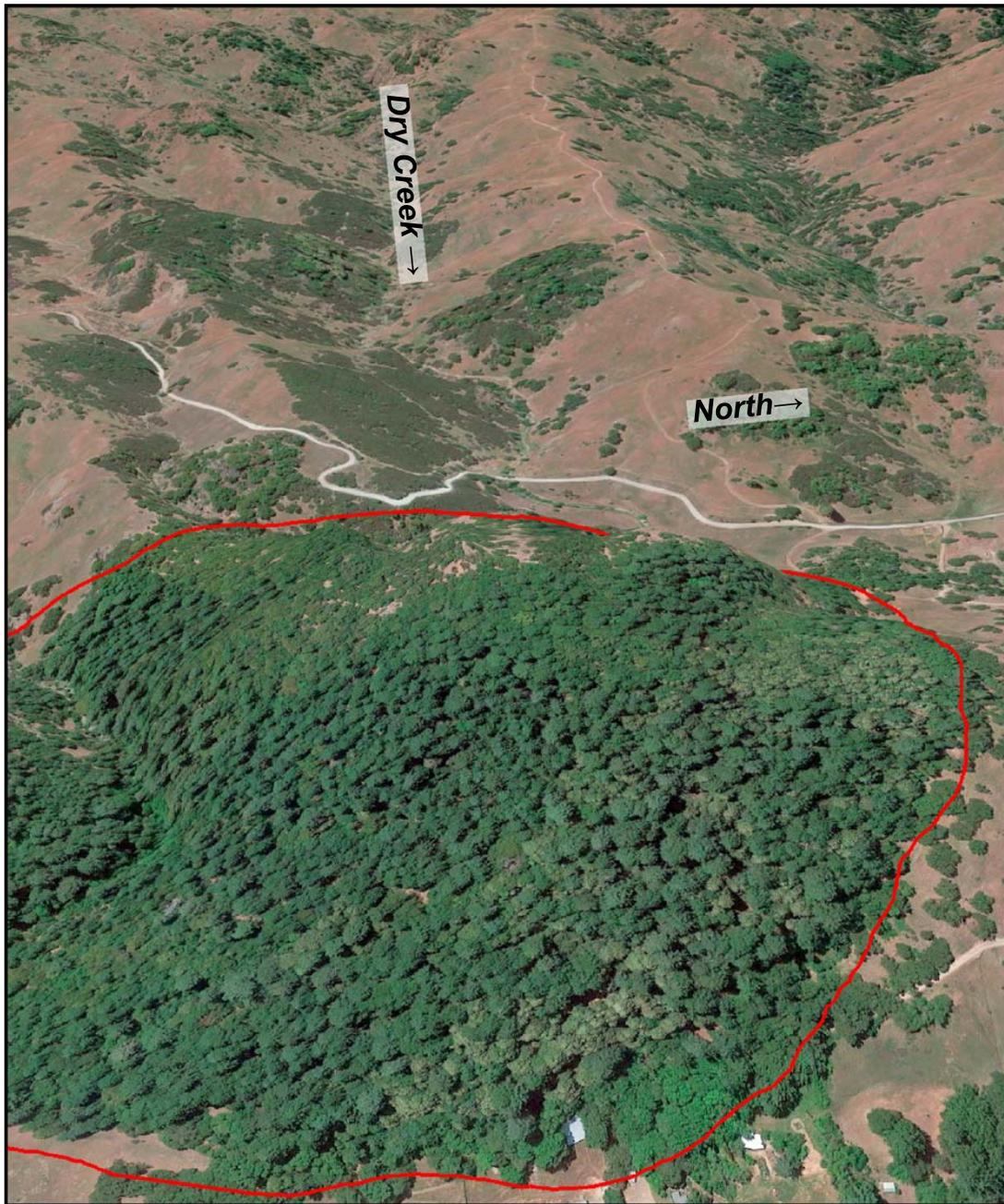
Figure 3.14: Perspective view near the mouth of Dry Creek at the Central Belt site. Red line denotes contact between sandstone block (covered with mixed broadleaf-needleleaf evergreen forest) and *mélange* matrix (with primarily annual herbaceous ground cover) from reconnaissance geologic mapping. Scale varies in this west-looking view; sandstone block is  $\sim 750$  m across in W-E direction. Google Earth imagery date 30 May 2014, eye-altitude 1.5 km,  $1.5\times$  vertical exaggeration.
